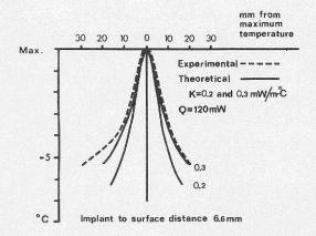
Fig. 5. Experimentally registered temperature profile over a 120 mW spherical heat source in a Perspex<sup>(R)</sup> plate at a distance of 6.6 mm from the surface, as compared to the corresponding theoretical profile over a point heat source in a material with a thermal conductivity of 0.2 and 0.3 W/m <sup>o</sup>C.
