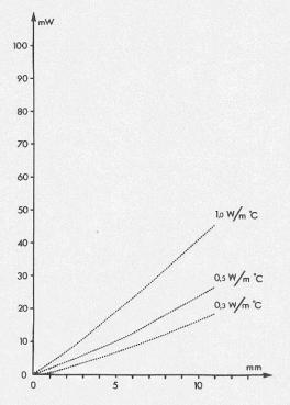
Fig. 6.b. Theoretical calculation of the heat production (ordinate) from a point heat source at increasing distance from the skin surface (abscissa), which should result in a 0.5 <sup>o</sup>C surface temperature increase immediately over the heat source. The calculation has been performed for three values of thermal conductivity of the surrounding tissue (0.3, 0.5, and 1.0 W/m <sup>o</sup>C).
