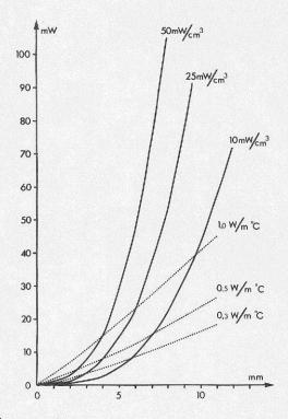
Fig. 6.c. Combination of Fig. 6.a and 6.b to give a theoretical illustration of the relation between possible (6.a, continuous lines) and necessary (6.b, interrupted lines) heat production from a buried heat source, resulting in a detectable surface temperature increase.
