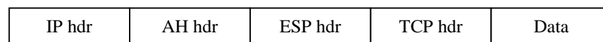
Figure 7.5: AH provides integrity to the ESP that in turn encrypts the transport payload.
