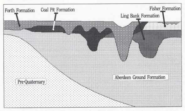
Fig. 4. Schematic section illustrating the relationships of seismostratigraphical formations in the British sector of the central North Sea in a transect from West to East. Horizontal distance c. 100 km. Total sediment thickness c. 250 m.
