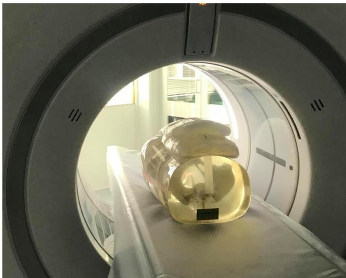
Figure 2. The pelvis phantom in the isocentre with the gels representing the second trimester.
