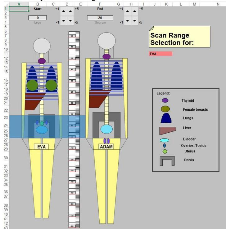
Figure 6. The female phantom to the left with a scan range over the pelvis area, the picture is a copy from the program (Stamm & Nagel, CT-Expo version 2.5, 2017)
