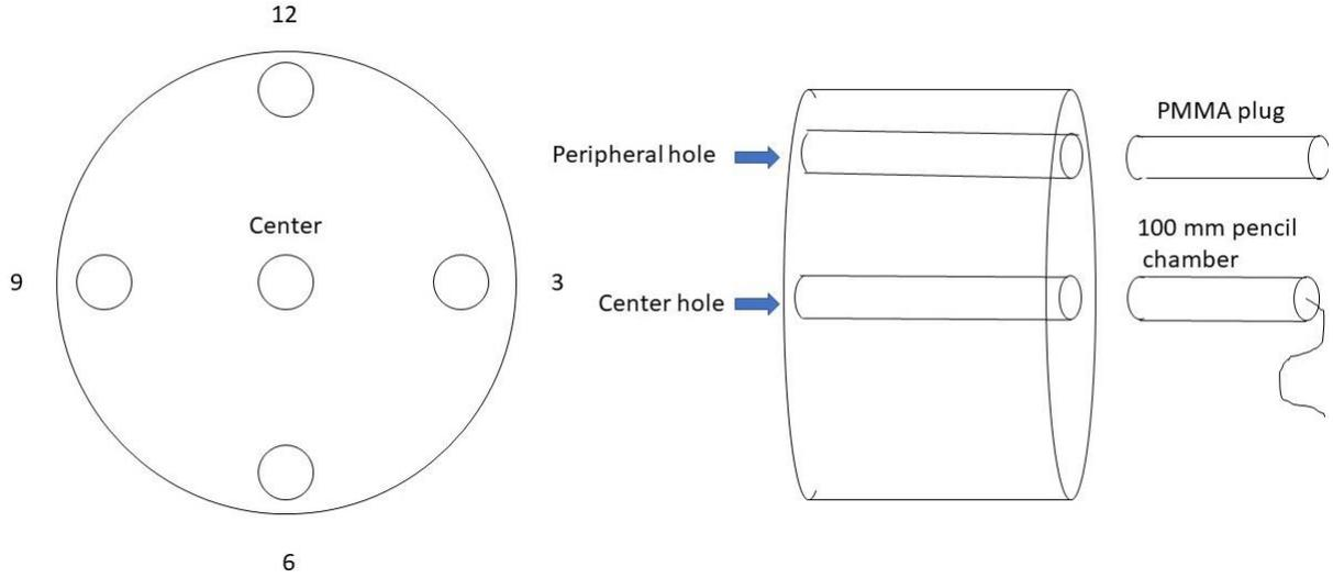
Figure 3. The general set up for the  $CTDI_{100}$  measurement in a standard CTDI PMMA phantom. There are two standard CTDI phantoms, 16 cm or 32 cm in diameter representing head or body respectively, both are 15 cm in length. The pencil chamber is 100 mm long and is placed either at the centre or at the periphery holes of the phantom. Unused holes may be plugged with PMMA rods. This picture is modified from an illustration in AAPM 204 (AAPM204, 2011).
