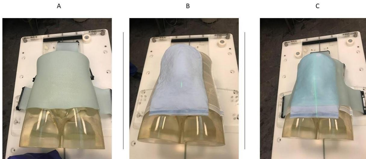
*Figure 1. The thermoplastic form for the second trimester under construction. A) show the base mould, B) shows the mouldable cushion formed into a belly on the pelvis phantom and C shows the top net laid on top of the cushion.*
