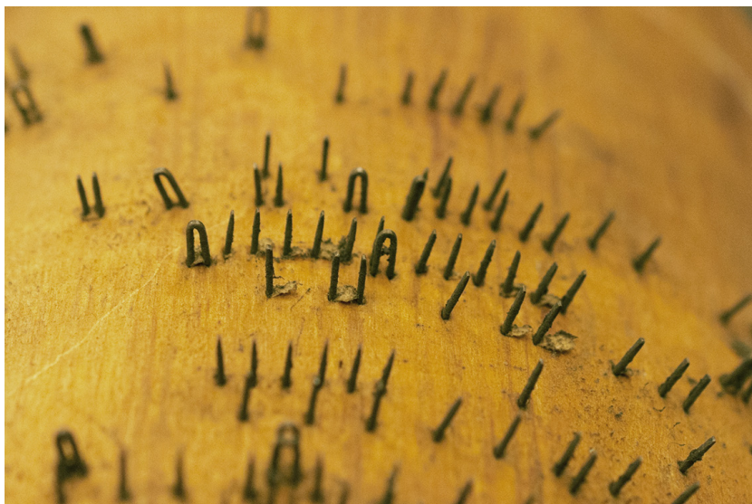
Figure 5. A pinned barrel belonging to the organ clock of the Royal Swedish Academy of Letters, History, and Antiquities, with traces of paper. Photo: Johan Norrback.
