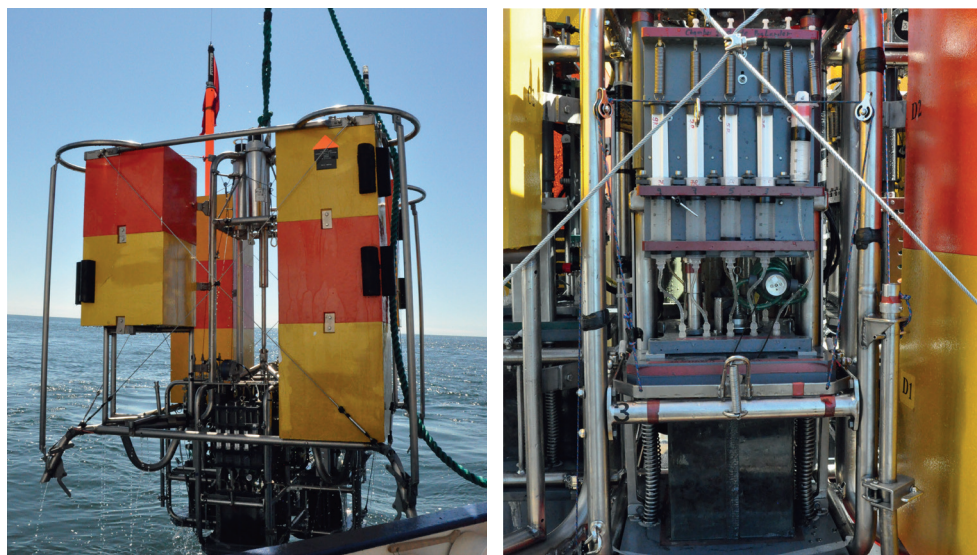
Figure 3 The big Gothenburg benthic lander at recovery (left) and a close up of the chamber module and attached syringes (right).
