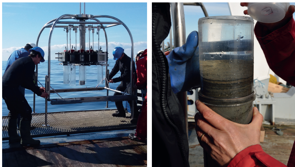
Figure 5 Multiple corer (left) that can take up to eight sediment cores (right). Tubes are 55 cm in length and 9.9 cm in inner-diameter.
